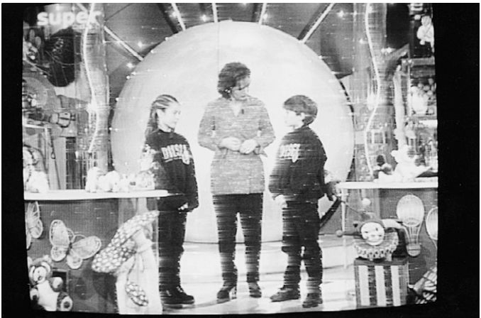
Fig. 4.8 Sparklies: the effect of noise in an f.m. picture transmission
