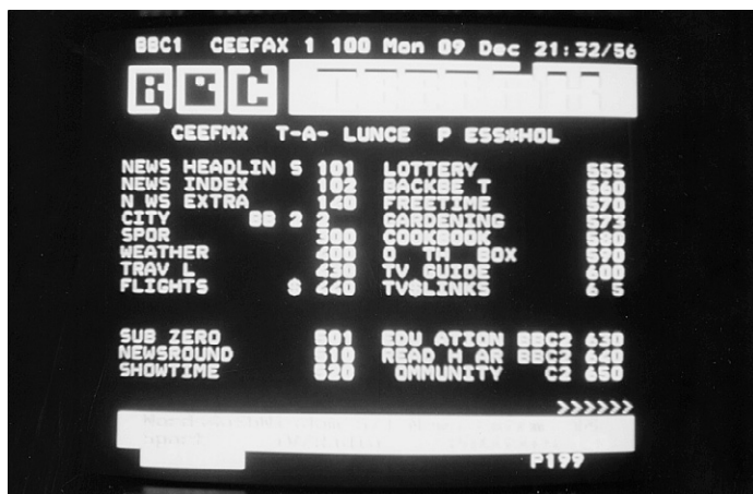
Figure 23.11 Severe corruption of a teletext page due to a badly damaged data pulse train
