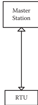
Figure 2.18 Single master–single remote configuration.
