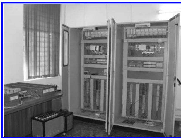
Figure 2.24 The DPU, RTU with I/O units.
