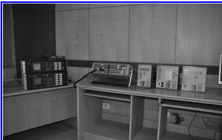
Figure 4.23 (See color insert.) The relay IEDs, secondary test device, and protocol converter.
