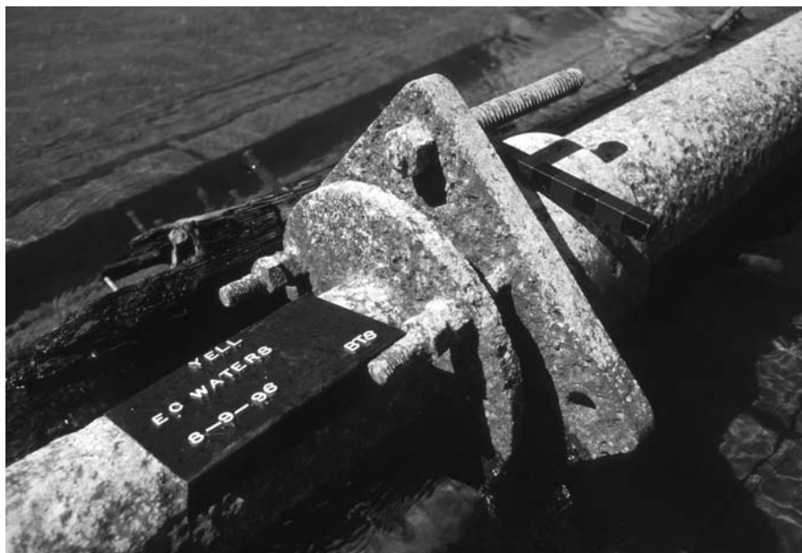
Fig. 2.61 View southwest of forward end of stern tube stuffing box and gland. Note large bolt on top that secured the shaft to the stern deadwood (now missing) through which it passed. Marked section of scale = 6 in. NPS photo by Brett Seymour
