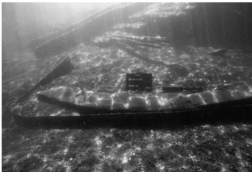
Fig. 2.74 Iron or steel strap near E. C. Waters ' stern. Scale = 1 ft. NPS photo by Brett Seymour
