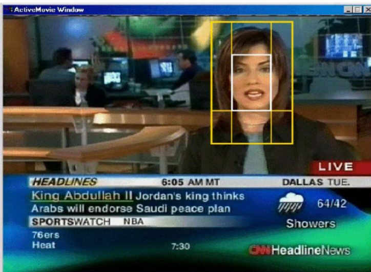
Figure 8.9. Face, with original (inside box) an expanded and partitioned (outside box) bounding box.
