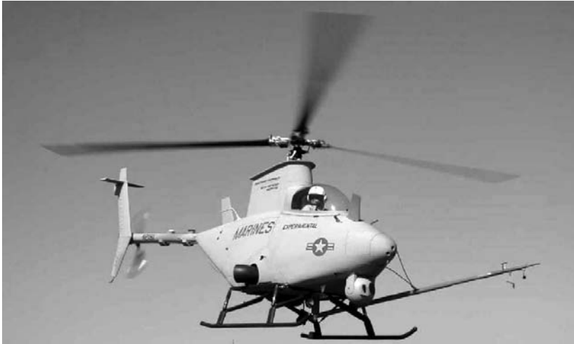
Fig. 13.14 Fire Scout P2 demonstrator — a variant of the Schweizer 333 (Northrop Grumman photo).
