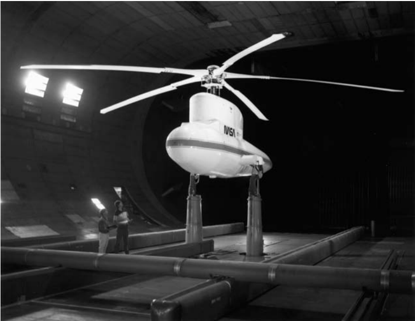
Fig. 5.15 Sikorsky bearingless main rotor (SBMR) test in the NASA Ames 40 × 80-ft subsonic wind tunnel.
