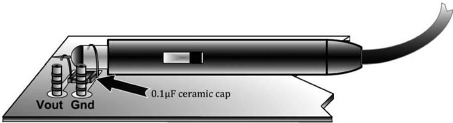
FIGURE 12.1 Correct way to measure noise and ripple.
