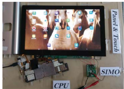
Figure 6.112 (a) 12-Inch tablet powered by the SIMO converter and (b) the whole tablet system, including the SIMO converter
