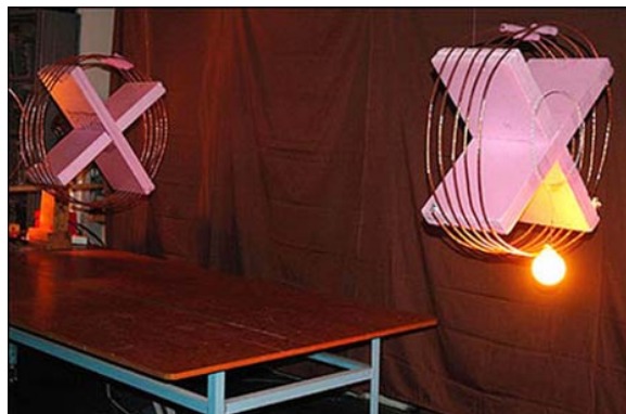
Figure 8.21 RF power transmission: MIT demonstration first showed how electricity can be wirelessly transferred to a device
