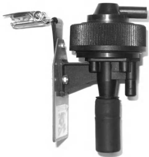
Figure 15.5 Conducting plastic personal respirable aerosol sampler.
