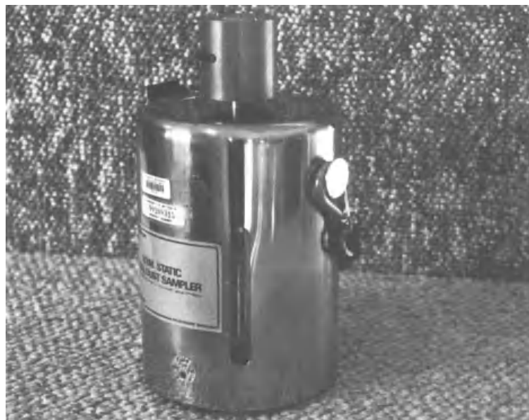
Figure 15.4 IOM static inhalable aerosol sampler.
