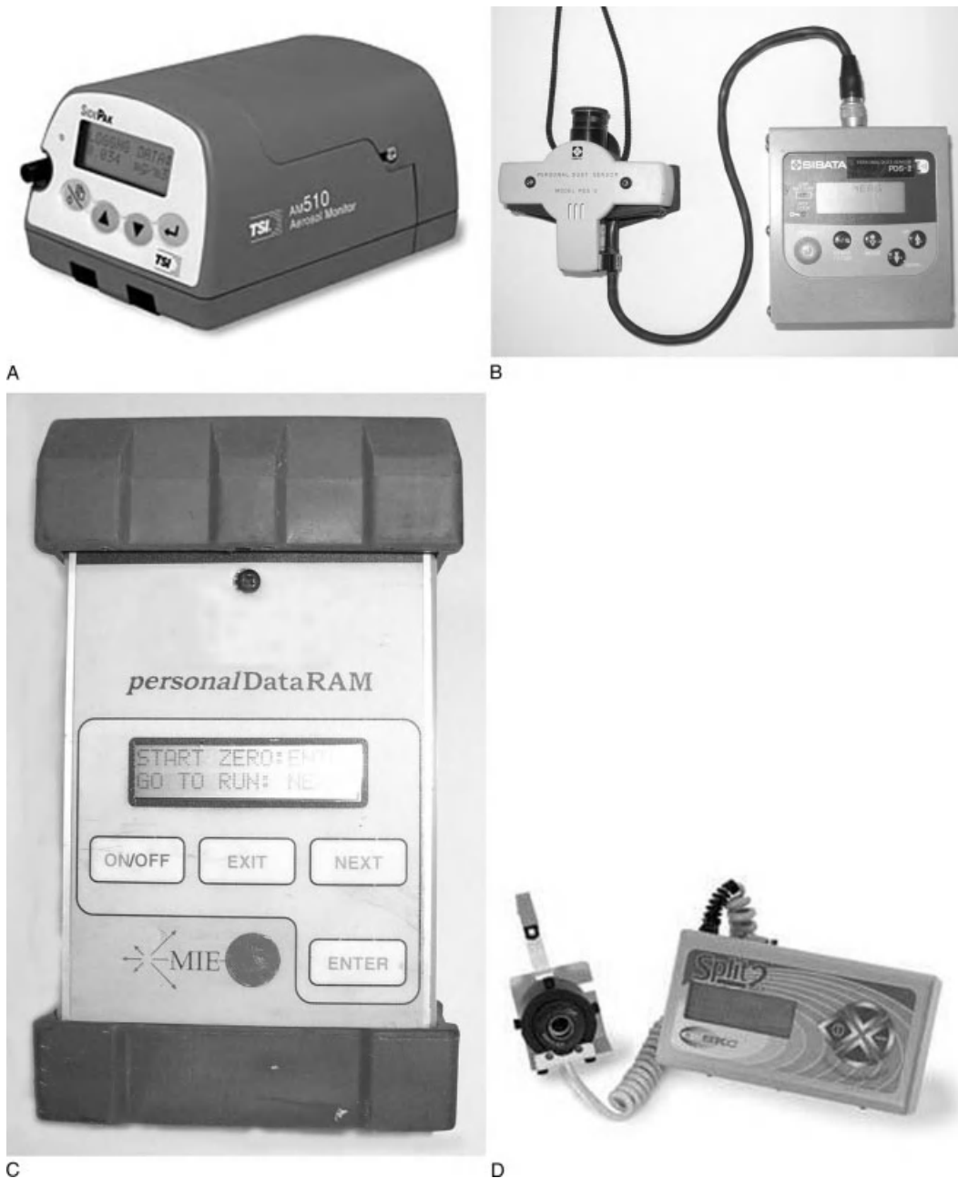
Figure 15.8 A selection of personal direct-reading aerosol monitors. (a) TSI Sidepak; (b) Sibata PDS1; (c) MIE personalDataRAM ; (d) SKC Split 2.
