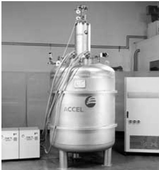
Figure 9.23. The view of the SMES device produced by ACCEL Instruments GmbH [24]
