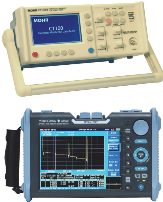
Figure 3.12. Time domain reflectometers (TDRs) for “copper” cables (left) and optical fibers (right)
