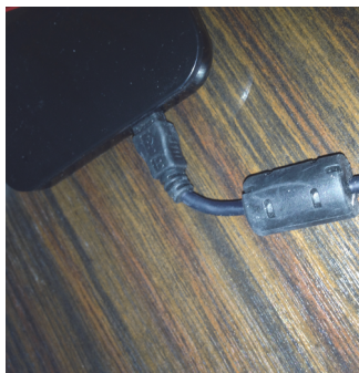
Figure 2.22. Common-mode filter of a USB cable
