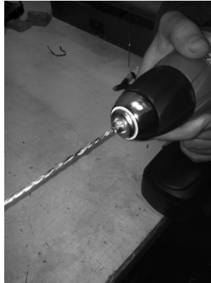
Figure 5.10. Economical production of a conductor with three isolated twisted strands
