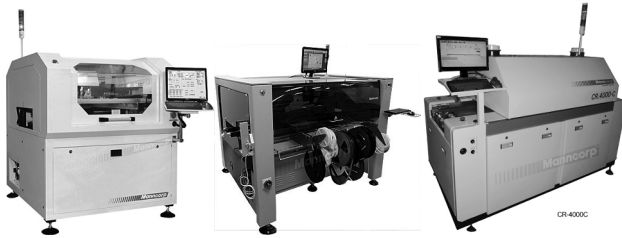
Figure 5.9. Paste application, component placing and reflow (Manncorp AP3000, MC-388, CR-4000C)
