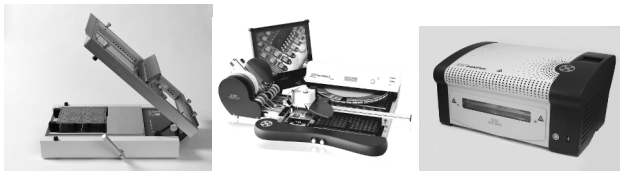
Figure 5.10. Paste stenciling (Eurocircuit eC-Stencil-Mate), component placing (LPKF Protoplace S) and reflow (LPKF Protoflow S)
