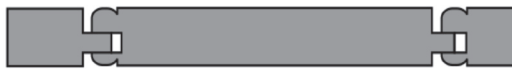
Figure 7-58. Tongue and groove slats are notoriously leaky and difficult to seal adequately or cost-effectively
