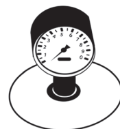
Figure 6-7. Blower Machine Gauge
