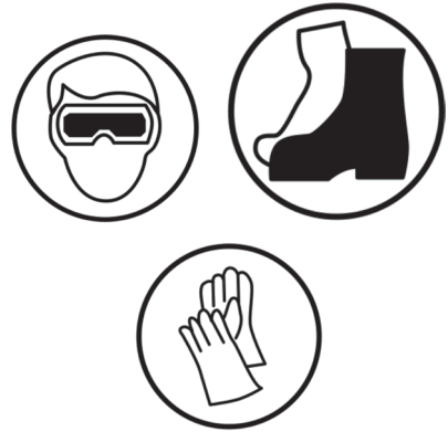
Figure 6-16. Safety glasses, steel toed shoes, and gloves are some of the basic safety tools that should be used almost all the time
