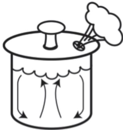
Figure 2-12. Convection of Water in a Hot Pot —Warm goes up. After it cools, it goes down.
