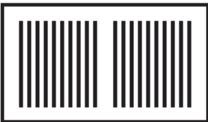
Figure 7-80. Vents like this should not be in garage walls.
