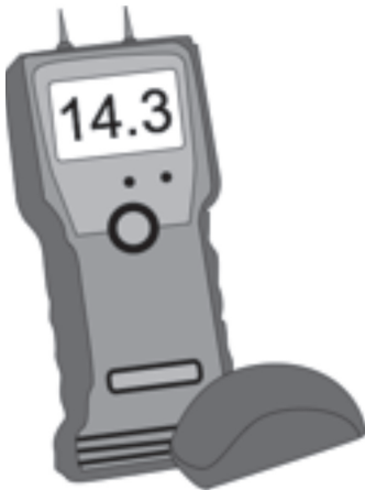
Figure 4-3. Moisture Meter. An electromagnetic version might look much the same but without the prongs.
