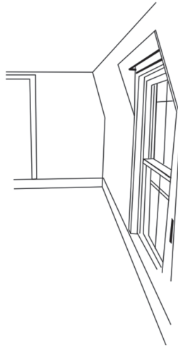
Figure 7-63. The “Wall” of a Mansard Roof From the Inside
