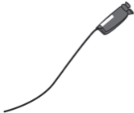
Figure 4-2. Borescope. A borescope is used for viewing into areas that are difficult to see, such as inside of walls, etc.
