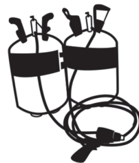
Figure 6-15. 2-Part Foam Tanks
