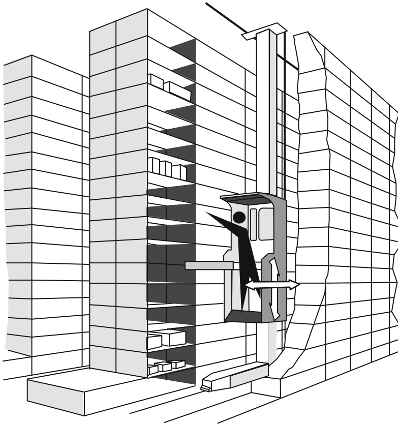
Fig. 6.51 Example of a commissioning system (Gudehus)
