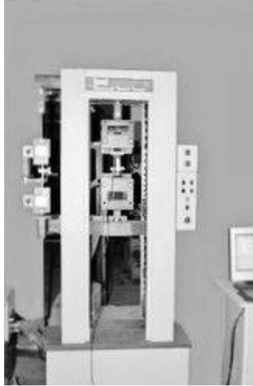
FIGURE 9.1 Wire rod, wire tensile and elongation testing unit.
