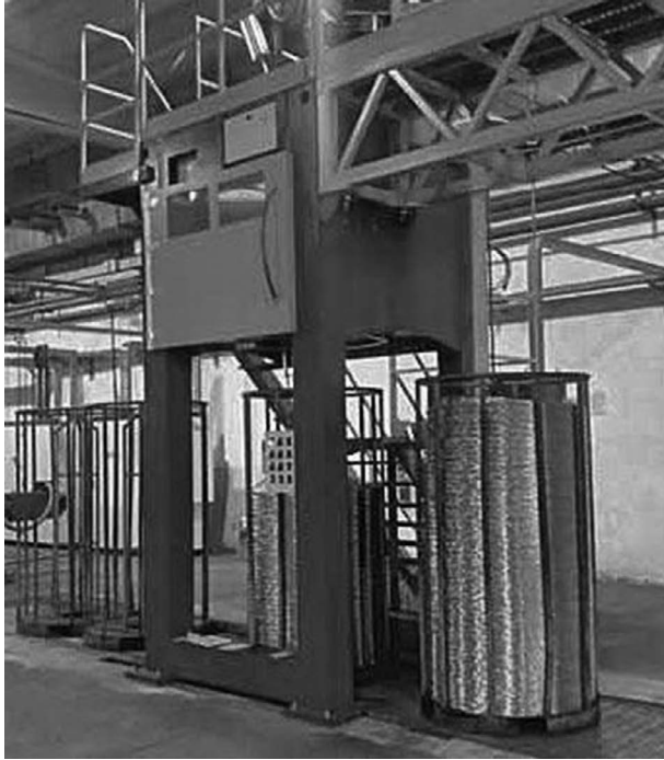
FIGURE 3.5 Basket coiler unit for copper and aluminium wire.
