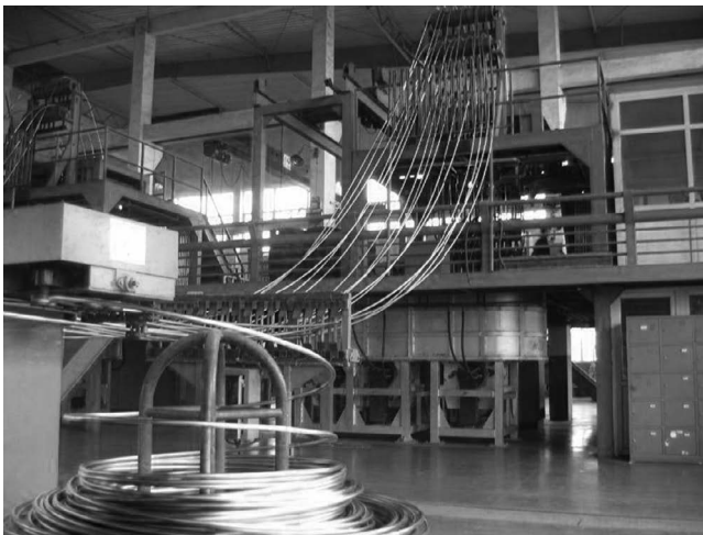
FIGURE 3.1 Up-cast unit for manufacturing copper wire rod.
