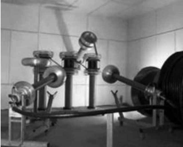
FIGURE 9.11 Shielded room for PD testing.
