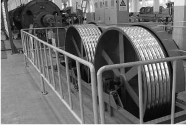
FIGURE 4.22 Stranding machine with guide plates, die holder box and dual groove–type capstan.
