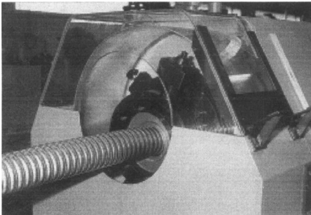
FIGURE 6.12 Corrugation unit of metal sheath: “UNIWEMA” machine.
