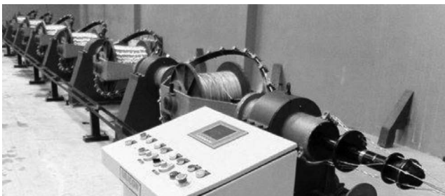
FIGURE 4.26 High-speed skip stranding machine, seven bobbins.
