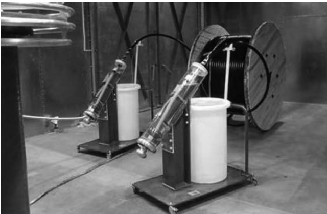
FIGURE 9.11 Shielded room for PD testing.
