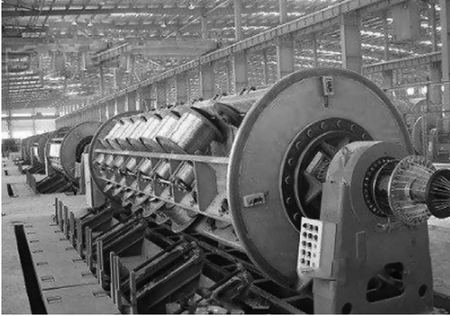
FIGURE 4.21 Rigid-type stranding machine with automatic batch loading system.
