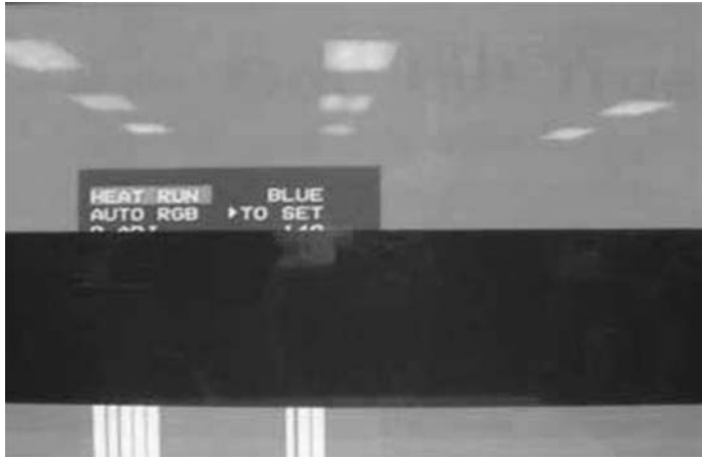
Figure 12.34: Symptom of a line gate driver fault
