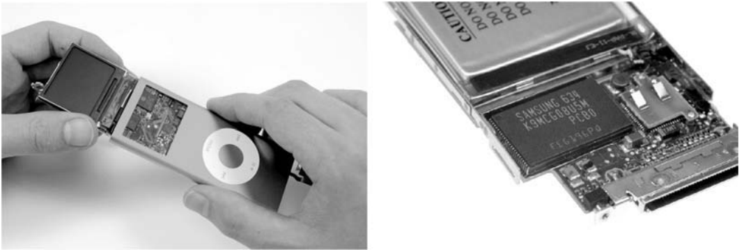
Figure 8.5: 8 GB iPod Nano teardown showing Flash memory storage 6
