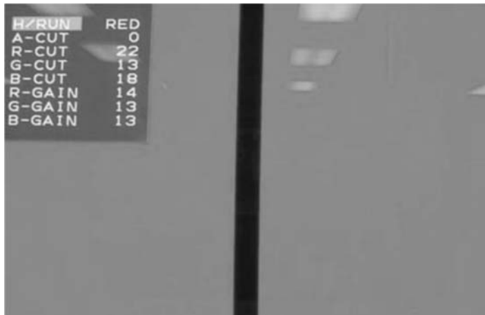
Figure 12.33: Source or column drive fault
