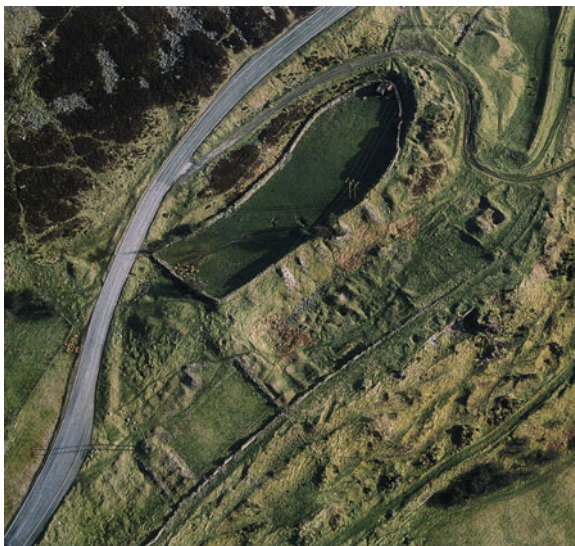
Fig. 10.2 Aerial view of the site of the Garnddyrys Rolling-mills at Blaenavon; the square at bottom left is surrounded by the foundations of key workers' housing on three sides. The oval on the upper picture is the former millpond for the mills that lay below it, and at the right-hand middle edge of the picture are the foundations and cellar of the works manager's house (Crown Copyright RCAHMW)
