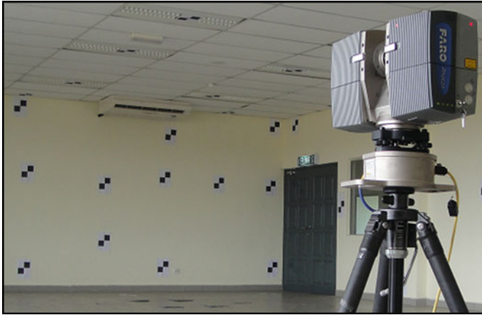
Fig. 11 Self-calibration for the Faro Photon 120 scanner
