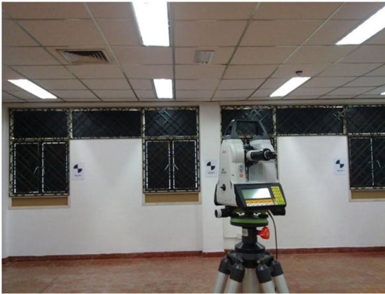
Fig. 4 High accuracy theodolite (Leica TM5100A)
