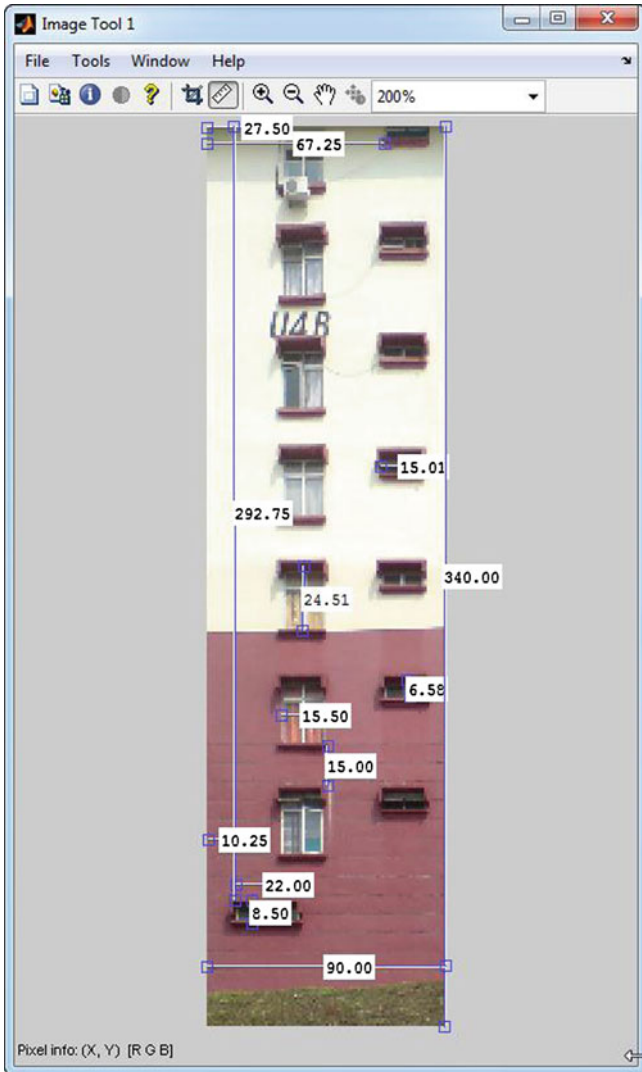
Fig. 4 Measuring all the required parameters for DPF via programming in Matlab
