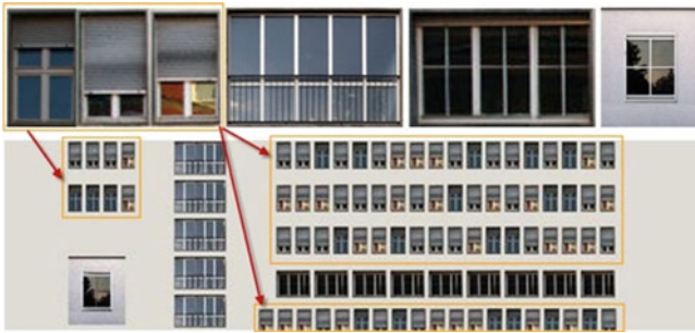
Fig. 3 One pixel is used for the wall texture and three random textures are used for three window layers to increase level of realism (LoR)
