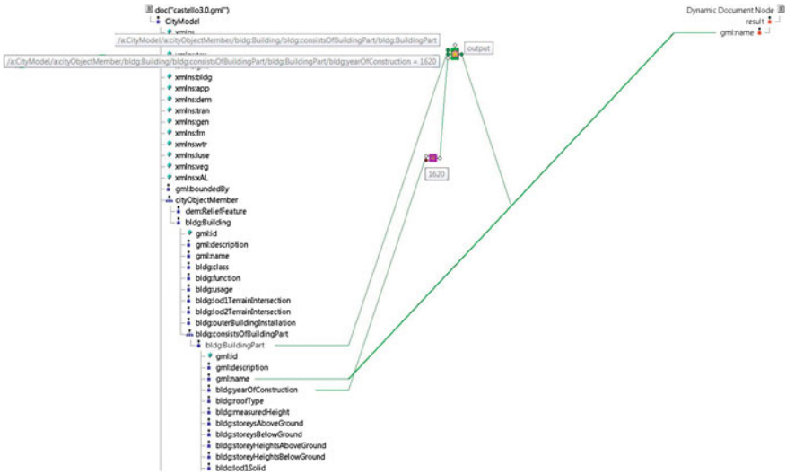
Fig. 8 Visual representation of the FLWOR operator: the Where clause in the magenta box defines the value (1620) of the yearOfConstruction attribute, while the others in the green box For (top) small Let (bottom) and Return (right) define the node list to be analysed, the variable association and the result to be shown
