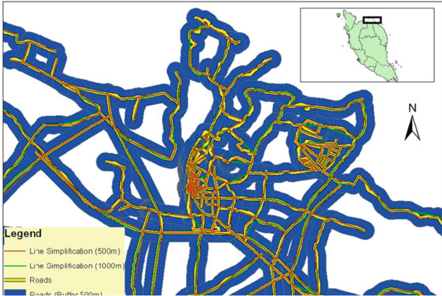
Fig. 10 A buffer zone is created around roads along with simplified transportation network (roads): original roads (yellow), simplified with different tolerance (red and green)
