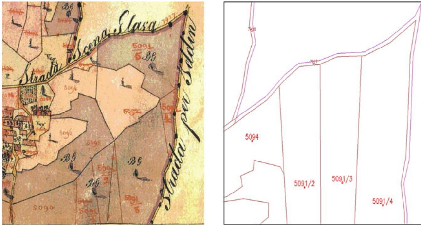
Fig. 2 Cadastral plans from different periods ( left middle of 19th century, right present day—electronic)
