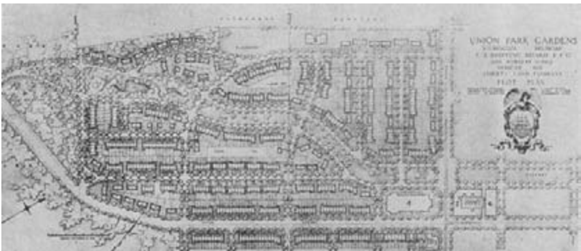
FIG. 2.5 Site plan for Union Park Gardens designed by John Nolan. Number 4 indicates the location of the community building. The size of the proposed structure suggests the importance of shared neighborhood facilities in the minds of the project's designers. Numbers 1, 2, and 3 mark apartment buildings. Number 5 labels the local school; Number 6, a parking garage. The plan shares a number of elements with Forest Hills Gardens, including winding, irregular streets and communal spaces designed to impart a sense of place. To cut down on road-building costs and increase green space, there are no alleys to the rear of houses. Also, no large thoroughfares cut the tract so as to reduce noise, pollution, and danger to children from traffic.
