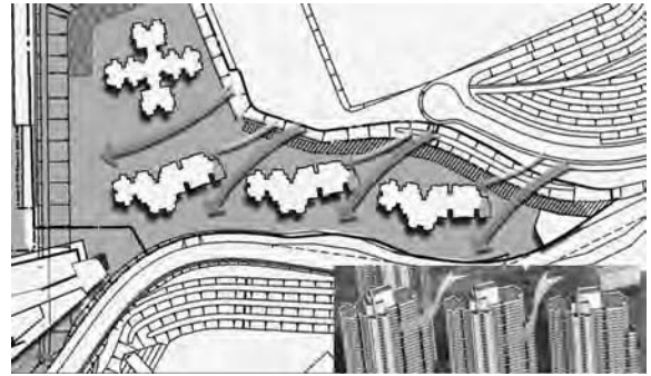
Note: For constrained sites of narrow linear configuration, design options for disposition and orientation (deviation up to 10°) of high-rise domestic blocks are compared in microclimate studies to streamline the wind flow across the development. The wind speed in the open spaces between domestic towers increases substantially by 100 to 133 per cent by adopting the master layout. This enhances the wind environment at the promenade in the front and attracts more social interaction and pedestrian circulation.
