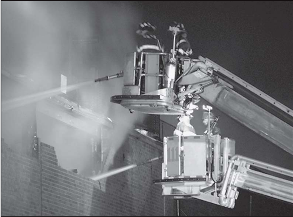
Fig. 17–1. Two tons of water delivered by master streams can cause a building collapse.
