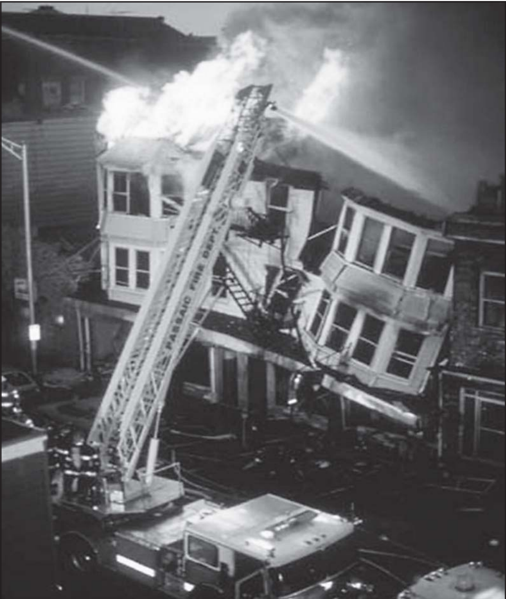
Fig. 18-3. Aerial devices cover the front and are positioned at the corner outside of the collapse zone.
