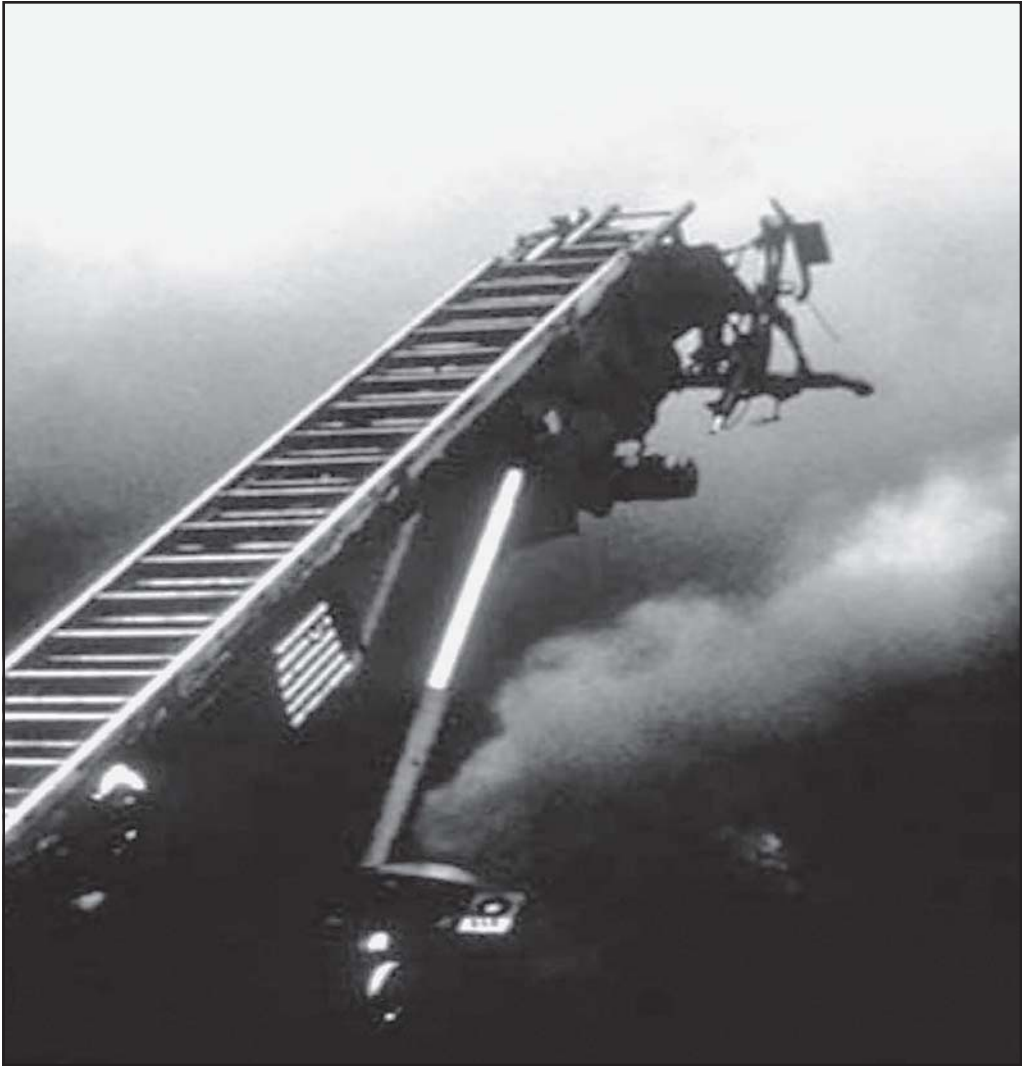
Fig. 17–2. This aerial master stream was operating in the collapse danger zone.
