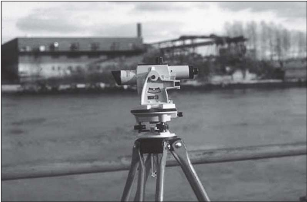
Fig. 18-11. A transit can monitor the slight movement of an unstable secondary collapse danger.
