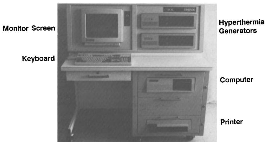
Figure 4. The conductive, interstitial hyperthermia system.
