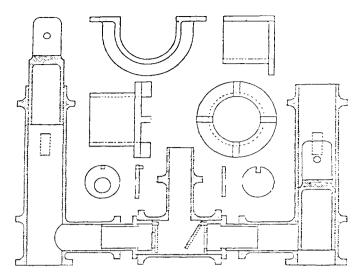
**Figure 23.1.** Diagram of a Roman pump found at Bolsena, in the British Museum, based on the work of Ctesibius of Alexandria, third century B.C, as published in G.V. Blackstone, *A History of the British Fire Service* (London: Routledge and Kegan Paul, 1957). Reprinted by permission from Routledge.
