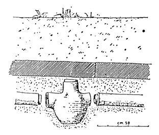
**Figure 16.12.** Section of settling basin, part of a waste water system, found at Syracuse. Published by Pace, 1935–38, and reprinted by permission of Società Editrice Dante Algheiri.
