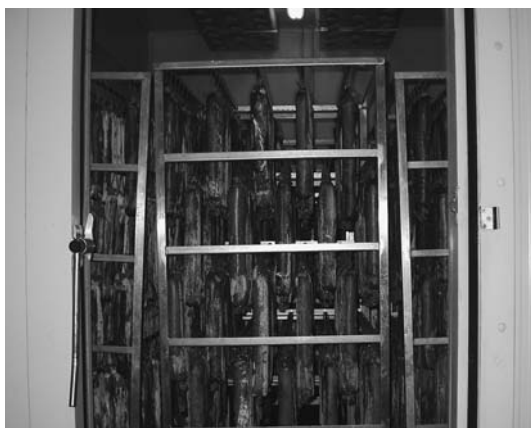
Figure 28.5. Example of a fermentation/drying chamber with computer control of temperature, relative humidity, and air flow rate. (By courtesy of Embutidos y Conservas Tabanera, Segovia, Spain.)
