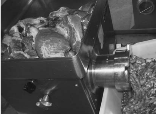
Figure 28.2. Grinding of meats and fats. There are many sizes of grinder plates in accordance to the required particle size.
