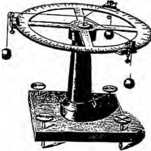
Figure 8.2 Varignon frame (taken from Alfred Weber's Theory of the Location of Industries , 1909, available at: www.csiss.org/classics/content/51 )
