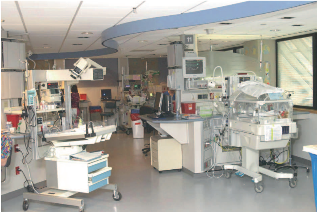
Fig. 8.3 The renovated NICU B has partial visual and auditory isolation of the staff and parents who are in the semi-closed bed spaces. At the time of the picture, the unit is 100% occupied. Note the acoustically dampening, translucent partition above the headwall and the muted south-facing exterior window in the upper right corner. The space in the view contains 7 caregivers, 11 babies, and 2 parents
