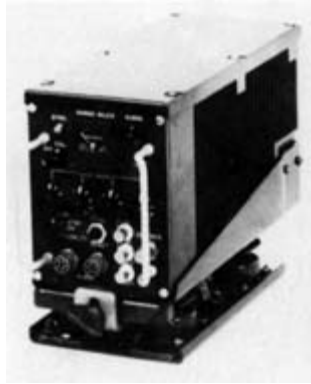
Figure 2.28(b). 1965 picture of the MX-118 applique, a member of the ARC-50 radio family and the first to use Gold codes. (Photo courtesy of Robert Dixon.)
