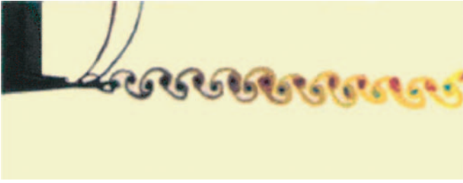
Plate XIV. Vortices structure behind a stationary NACA 0012 (Lai and Platzer, 1999).
