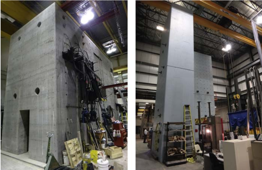
Figure 26.7 Two of the strong walls in the Department of Civil Engineering at the Université of Sherbrooke.
