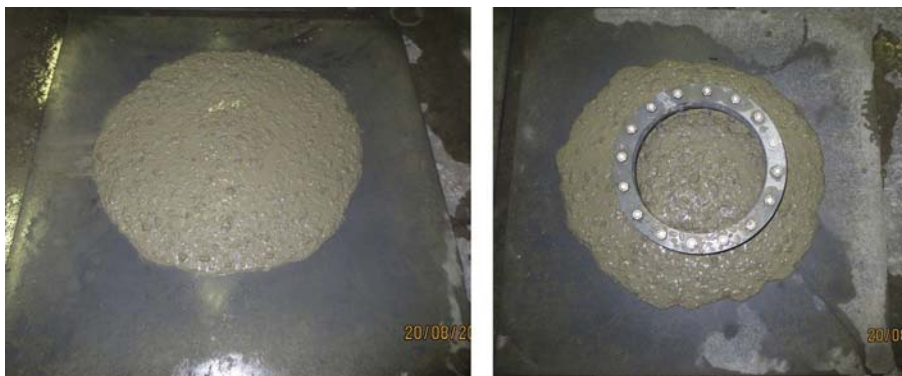
Figure 26.2 Measuring passing ability with a J-ring.
