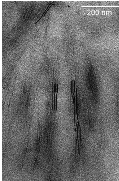
Figure 10.7 TEM image of a poly(methacrylate-g-PEO)/hydrocalumite composite. Lines are drawn as guides for the eye. The interlayer spacing measured between those lines varies between 7 and 10 nm.
