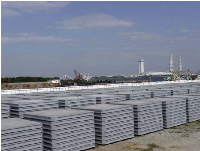
Figure 27.21 The UHSC slabs stocked in the plant yard.
