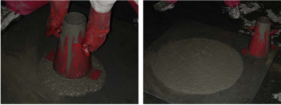
Figure 26.1 Slump flow measurement.
