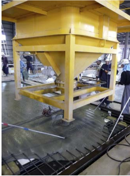
Figure 27.20 The filling of the moulds with UHSC.
