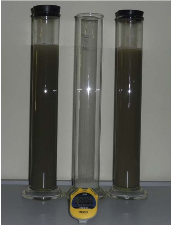
Figure 1 Sedimentation of cement particles with and without a superplasticizer at time t = 0 . The suspension is then left to settle.
