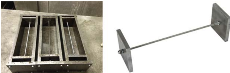
Figure 22.7 Typical molds used to measure the restrained expansion according to ASTM C878 standard procedure (Aïssi et al., 2014).
