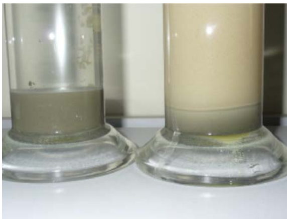
Figure 4 Close view of the bottom of the two graduated cylinders after 24 h: without superplasticizer (left) and with superplasticizer (right).
