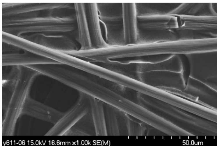
FIGURE 2.9 SEM image of carbon paper (Toray, TGPH-090) pretreated with 20% PTFE [2].
