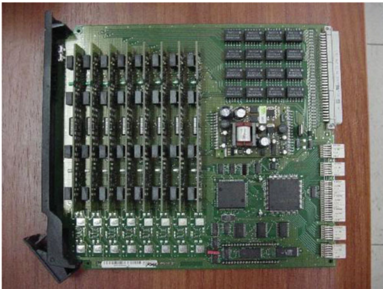
Fig. 3.11 A PBX board serving 32 digital sets
