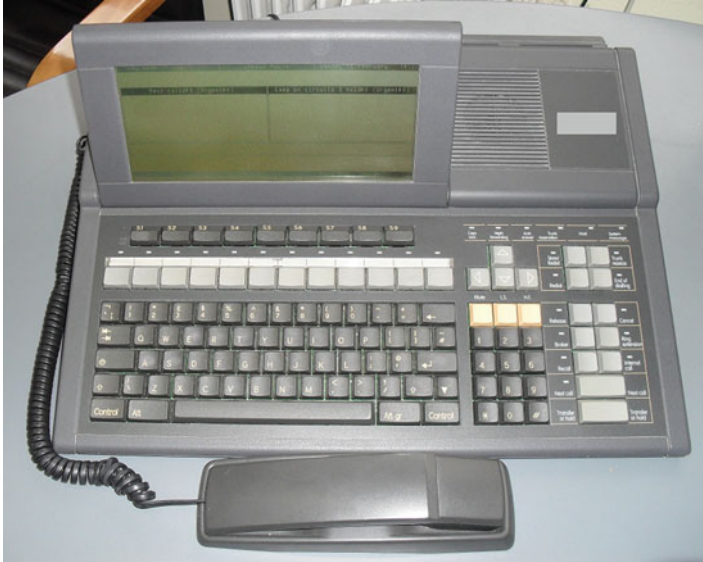
Fig. 3.14 A typical PBX operator's console
