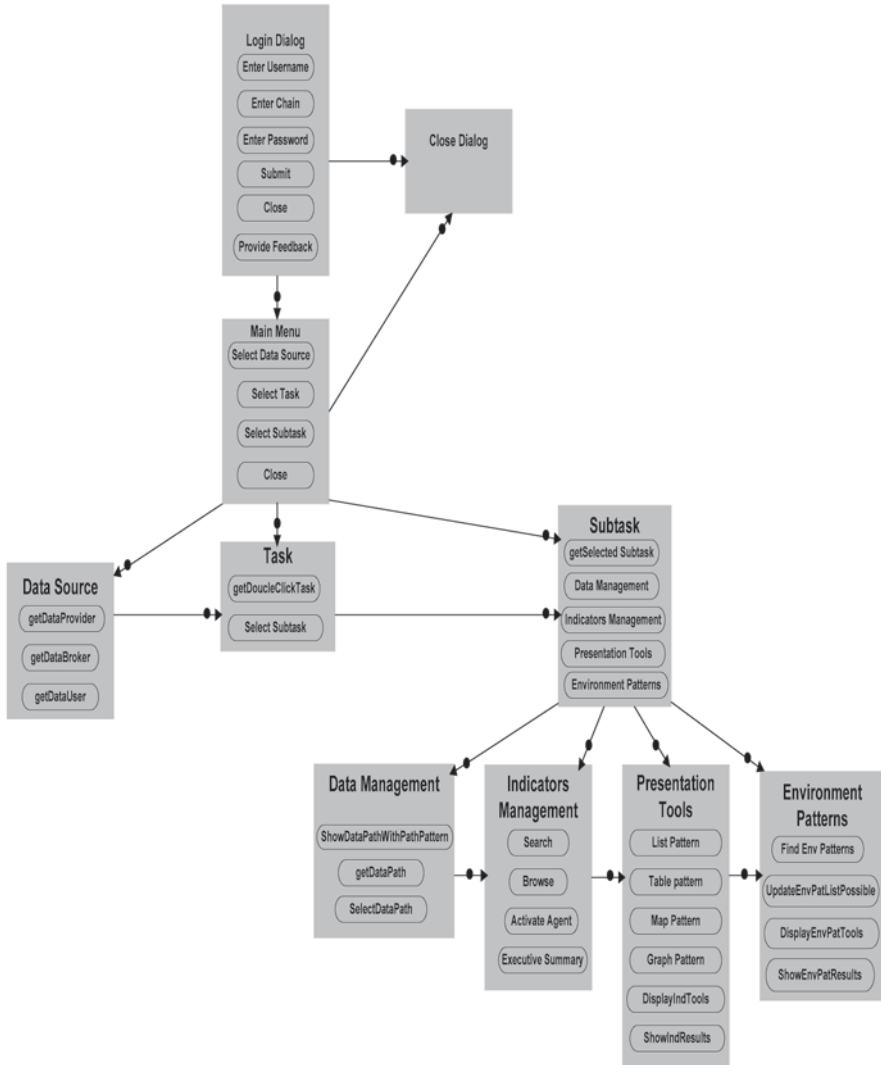
Fig. 9.17 Dialog graph of the environmental management interactive system for laptop and PDA platforms
