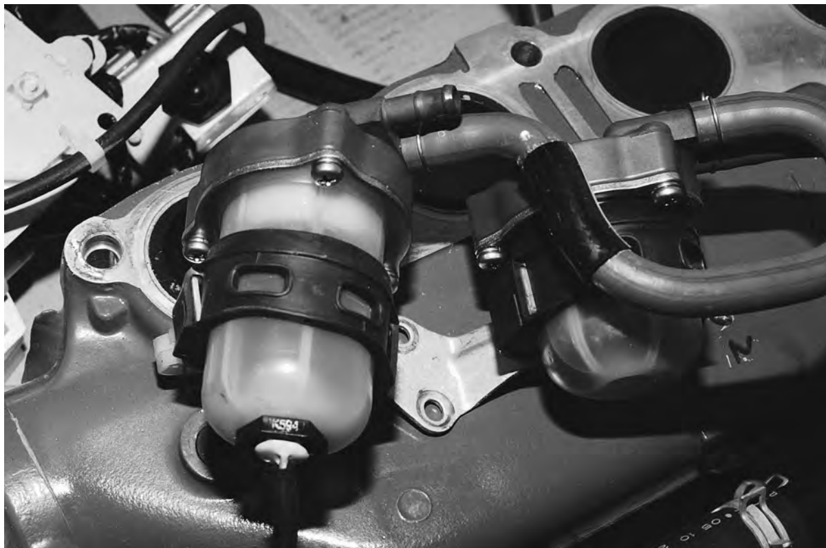
Figure 7-3. A fuel pump strainer mounted on a new Honda. Note the wiring sensor that warns of water.
