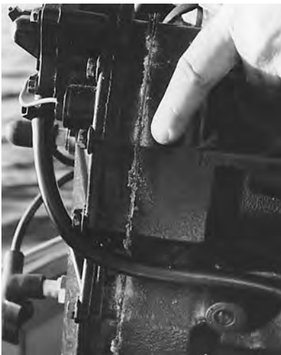
Figure 4-3. Head gasket beginning to leak—note corrosion at the joint.
