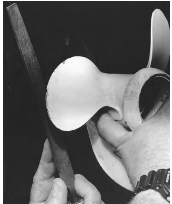
Figure 3-7. Filing out a nick in a propeller.
