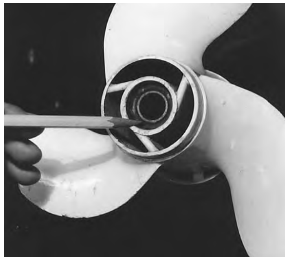
Figure 3-8. Vulcanized propeller hub being inspected.
