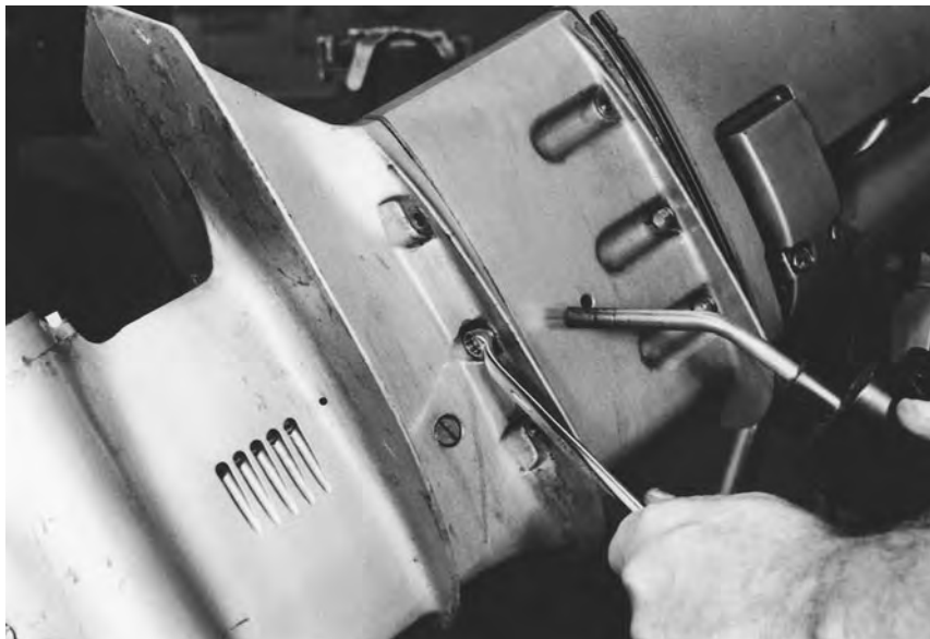
Figure 10-10. Applying heat and pressure to remove a frozen bolt.
