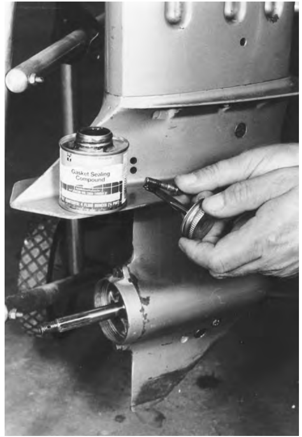
Figure 10-9. Coating a bolt from the lower unit with gasket sealer to prevent corrosion.
