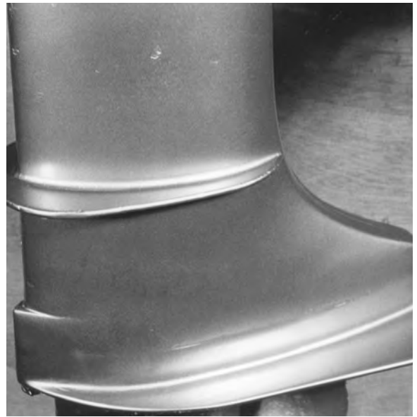
Figure 10-7. The corroded area completely refinished.
