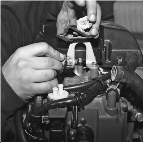
Figure 3-15. Thermostat removed for cleaning and inspection.
