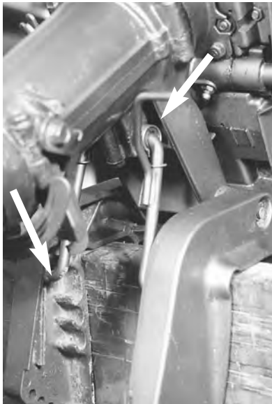
Figure 8-11. Lubrication points on a manual tilt mechanism.
