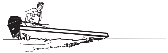
Figure 8-12. Boat and motor with too much “in” trim.
