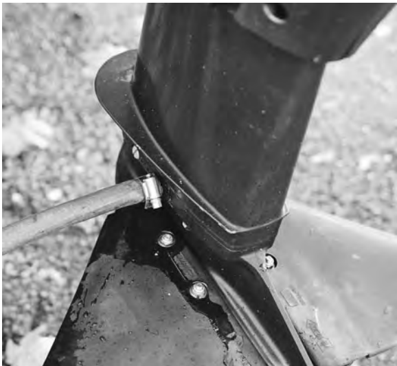
Figure 3-13. Hose attached for flushing the cooling system.
