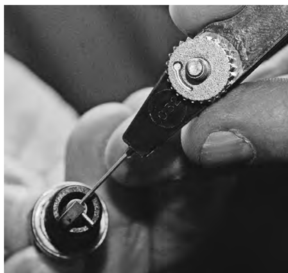
Figure 5-5. Using a spark plug gapping tool.
