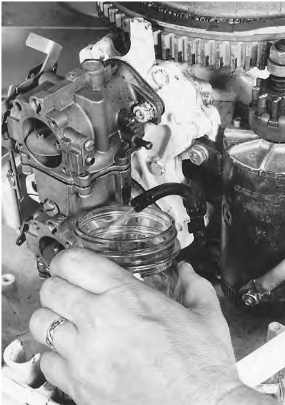
Figure 4-2. Checking that fuel is reaching the carburetor.
