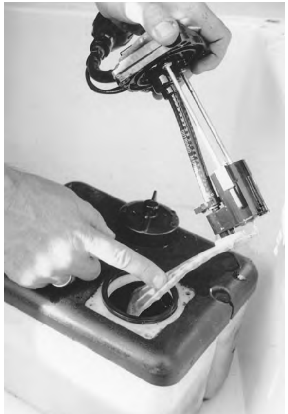
Figure 7-16. Inspecting the oil reservoir filter screen.
