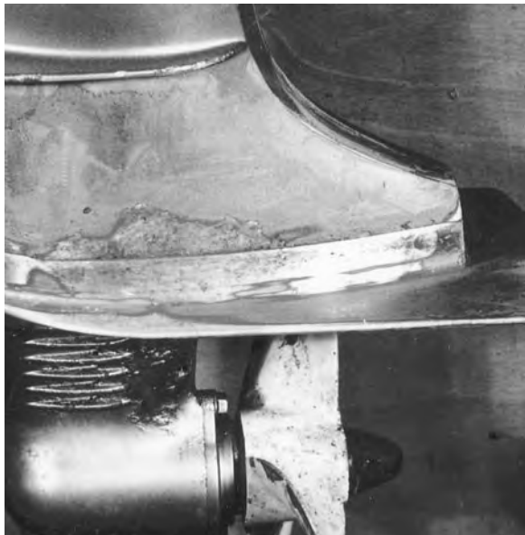
Figure 10-4. Corroded area sanded and ready for inspection.
