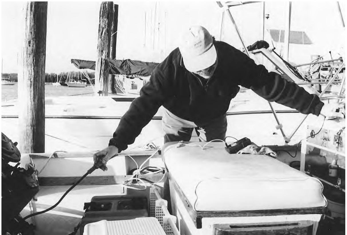
Figure 6-13. Extension harness ohmmeter test.
