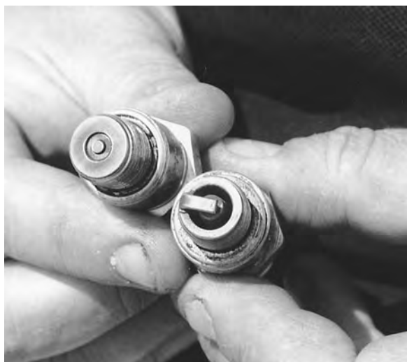
Figure 5-4. A surface-gap spark plug (left) and a conventional plug.
