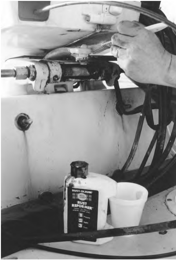
Figure 10-8. Applying “Rust Reformer” to part of the outboard engine.
