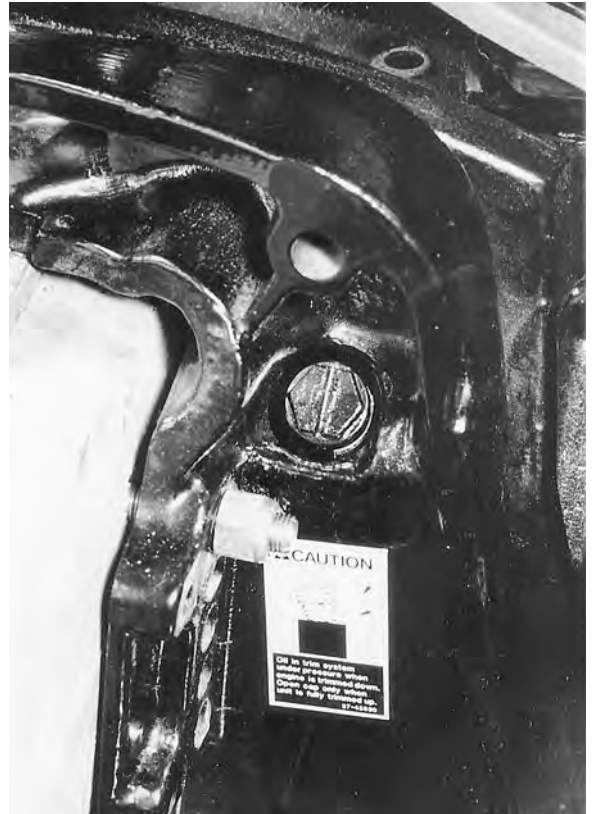
Figure 8-17. Typical hydraulic fluid fill cap for the trim and tilt system. This one is on a midsize Mercury engine.
