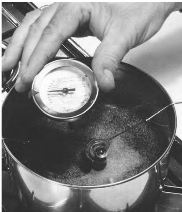
Figure 9-3. Testing a thermostat on the stove top.
