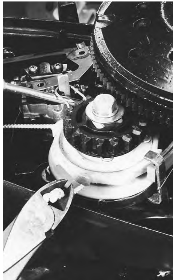
Figure 6-16. Removing a broken pull cord.
