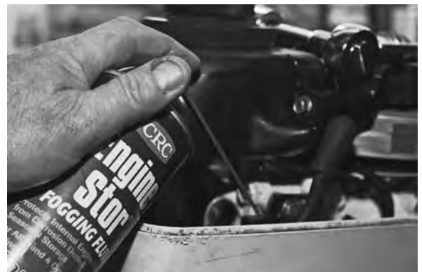
Figure 3-21. Spraying fogging oil into carburetor intake.
