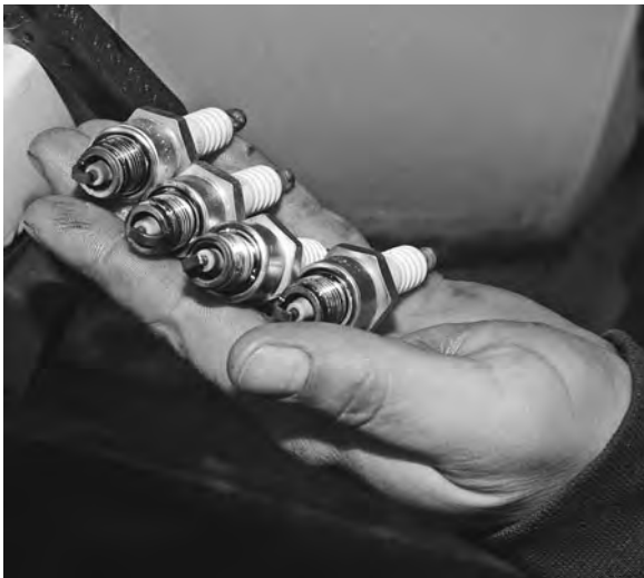
Figure 5-8. Properly burning spark plugs look like these. They should have a light-brown center electrode insulator, with a light fluffy black color around the perimeter of the plug.
