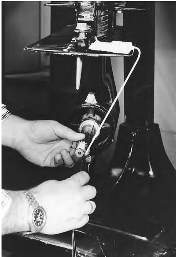
Figure 9-9. Checking for propeller-shaft run-out.
