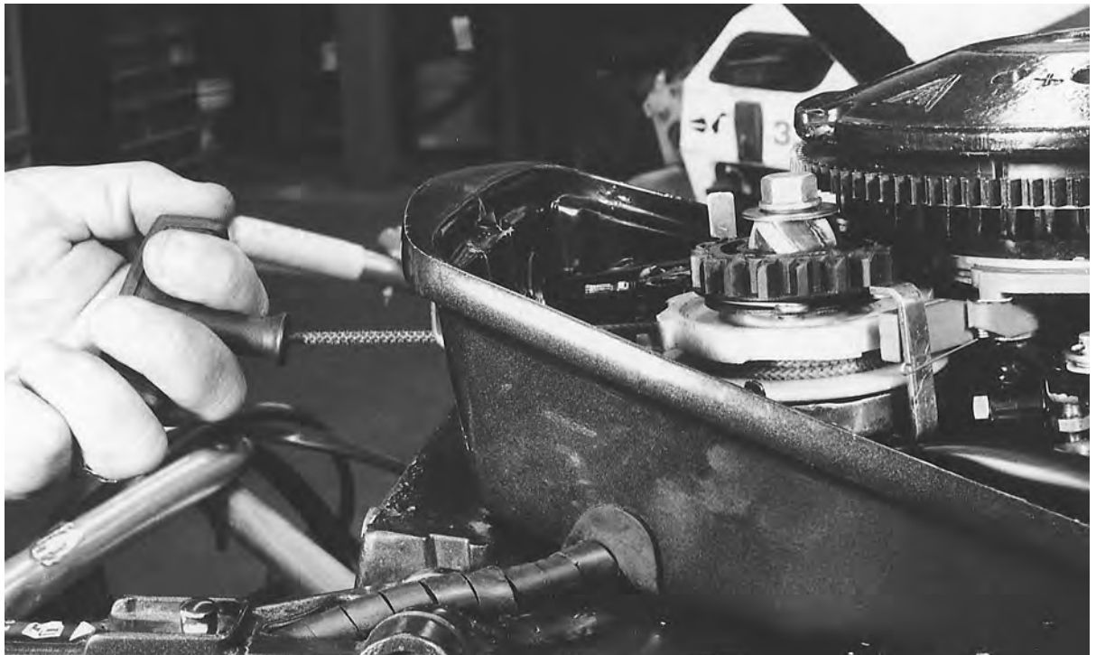
Figure 6-18. Winding on a new pull cord.
