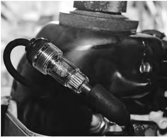
Figure 5-6. The neon tester in place and ready to use.
