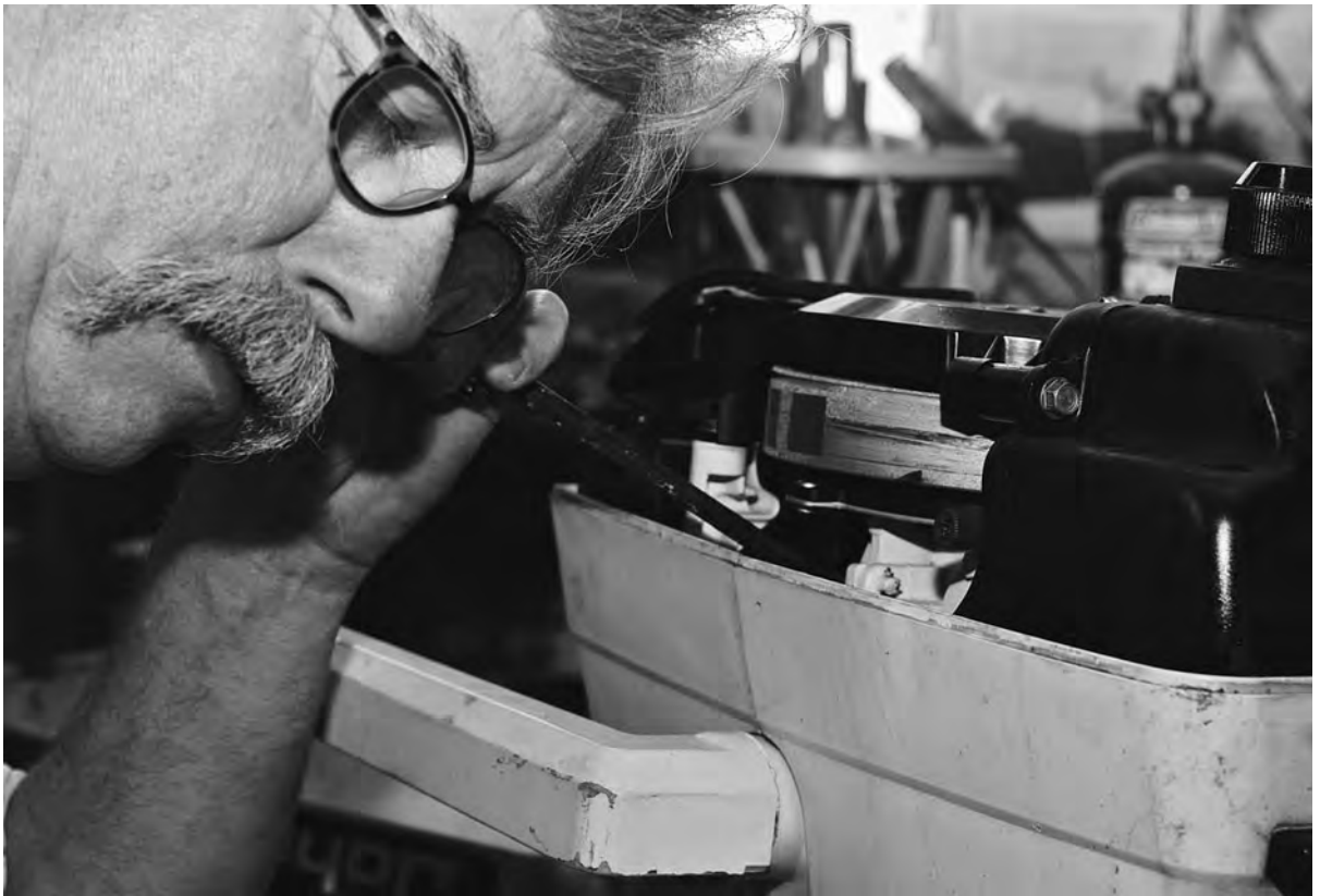
Figure 4-1. Using a screwdriver to pinpoint noises.
