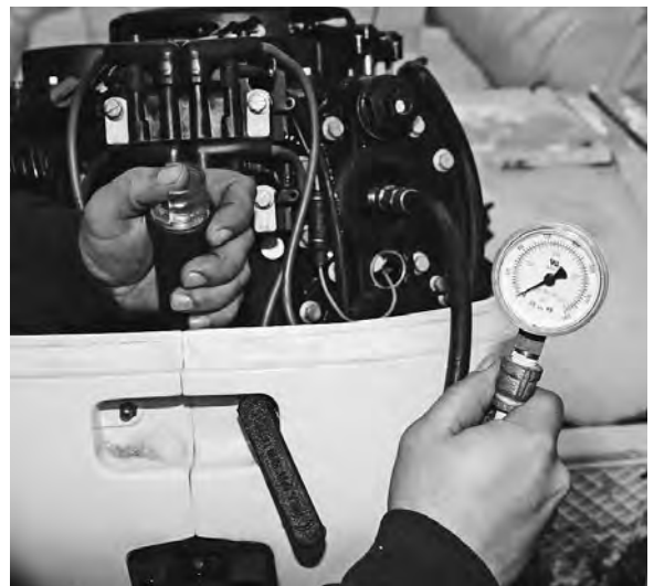
Figure 3-16. A compression test in progress.
