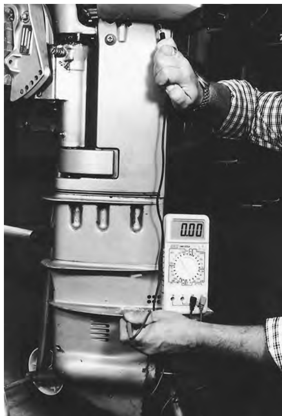
Figure 10-2. Using an ohmmeter to test continuity between a zinc and the engine case.
