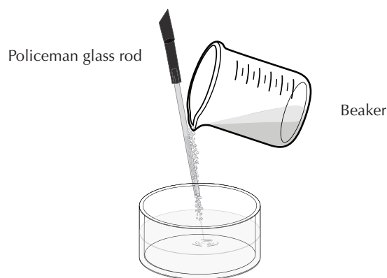
Figure 4.5: Policeman rod used for transferring liquids.
