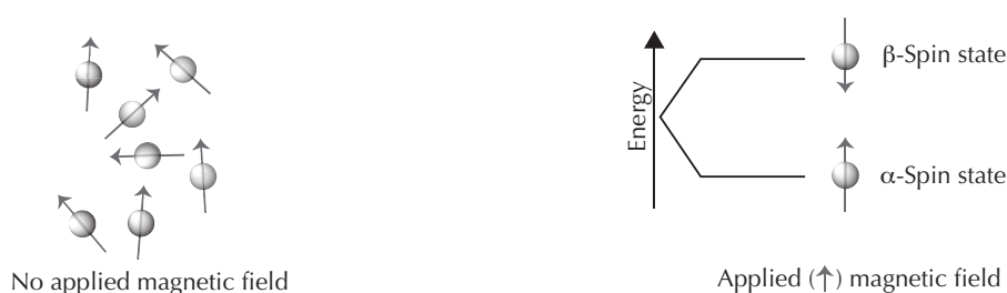
Figure 5.9: Orientations of nuclei when a magnetic field is applied.
