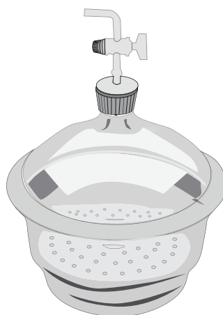
Figure 4.19: Desiccator for drying solids.
