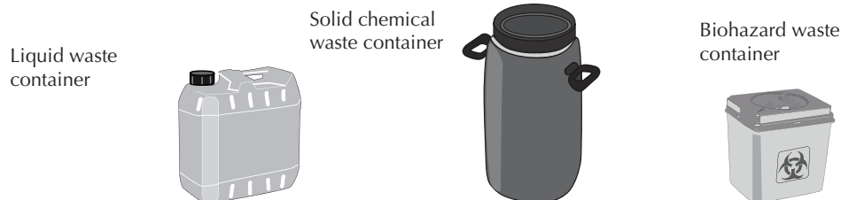
Figure 1.4: Different types of containers for waste storage.
