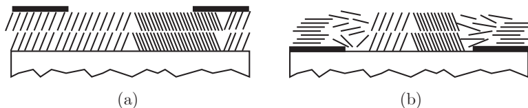
Fig. 5.3. A schematic illustration of the molecular packing in (a) top and (b) bottom contact OFET devices. Small molecules deposited on metal contacts tend to lie flat, and do not have a contiguous grain structure where the molecules are standing vertically at the center of the channel.
