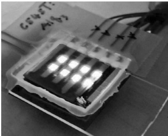
FIGURE 5.11 Top view of a structurally integrated OLED/sensor film/PD probe in a back detection geometry. (See also color insert.)
