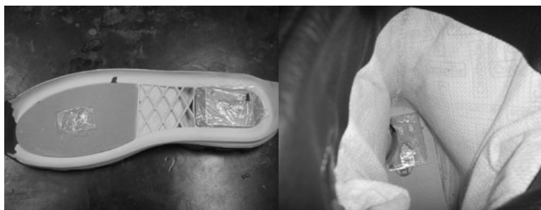
FIGURE 3.27 Experimental setup for detection of falls and gait analysis.
