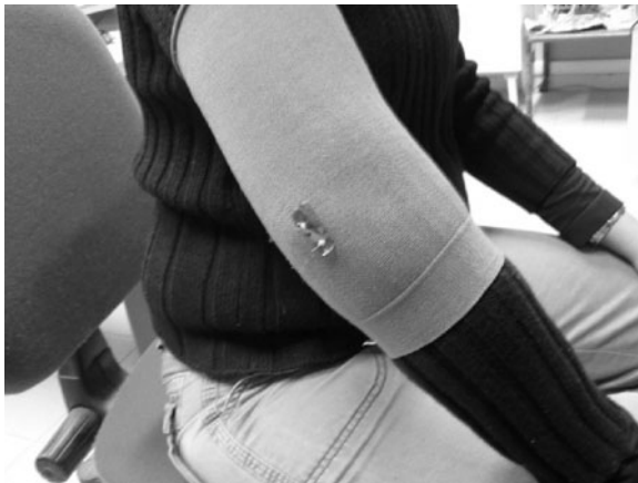
FIGURE 3.22 Application of a field-effect strain sensor to the elbow joint bending detection.
