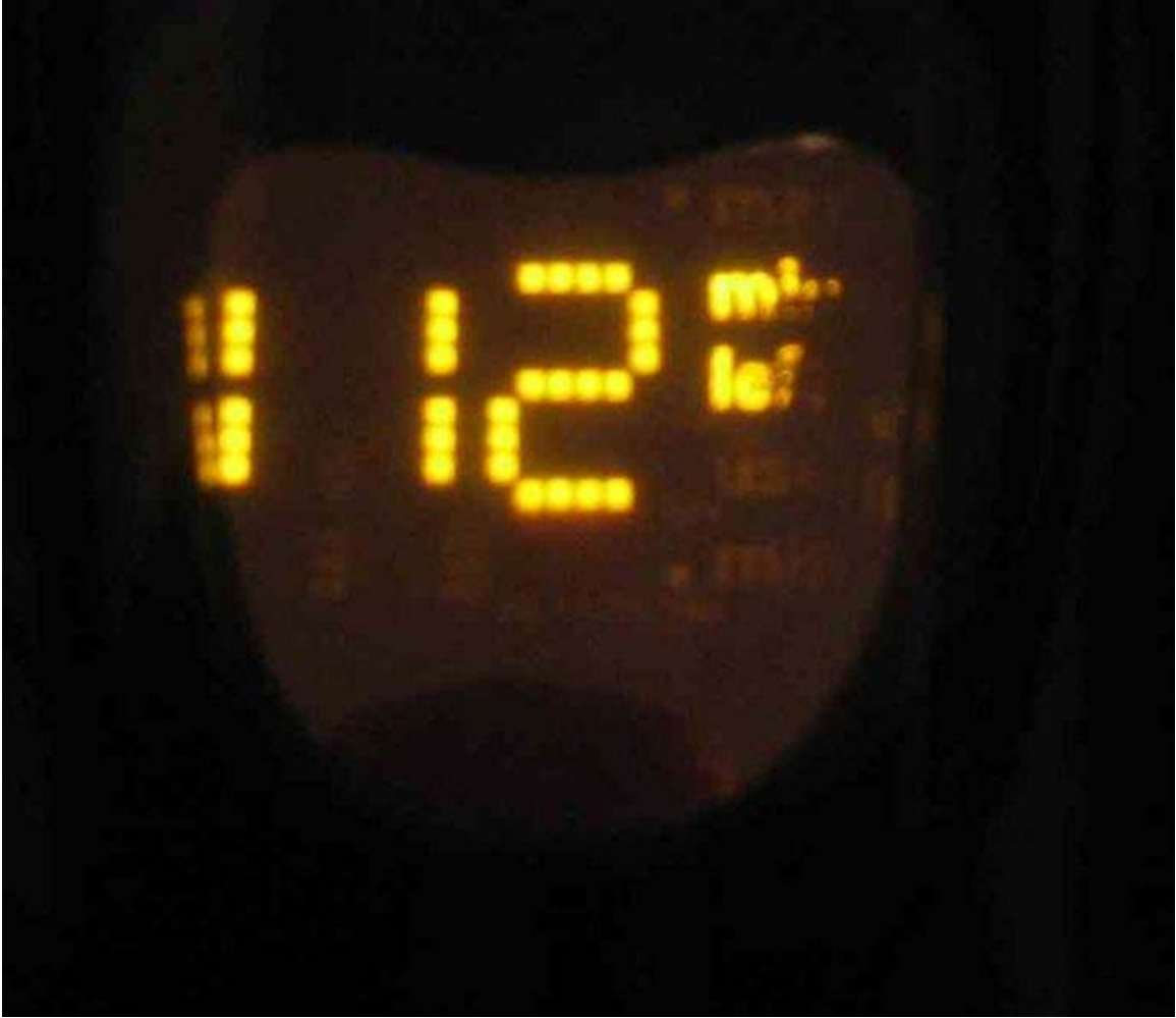
LEP display showing partial failure
