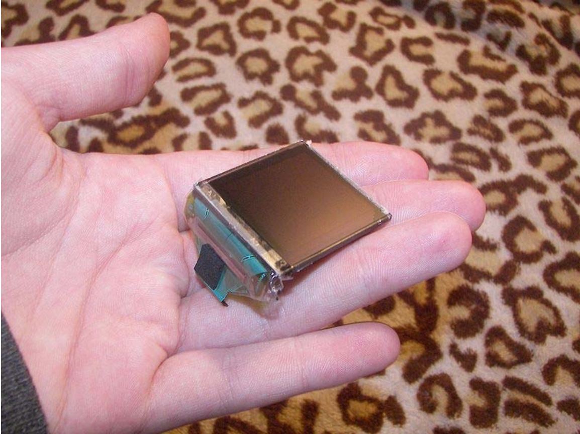
A 3.8 cm (1.5 in) OLED display from a Creative ZEN V media player
