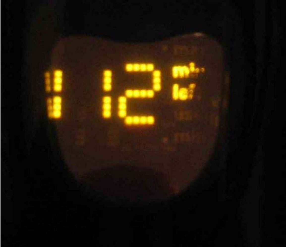
LEP display showing partial failure
