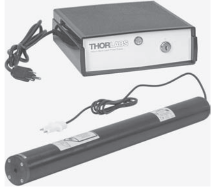
A modern He-Ne laser with its power supply. This unit provides a linearly polarized TE_{00} output at 633 nm (red) at a power of 10 mW. The beam diameter is 0.68 mm and the divergence is 1.2 mrd. The longitudinal mode separation is 320 MHz. (Courtesy of Thorlabs.)
