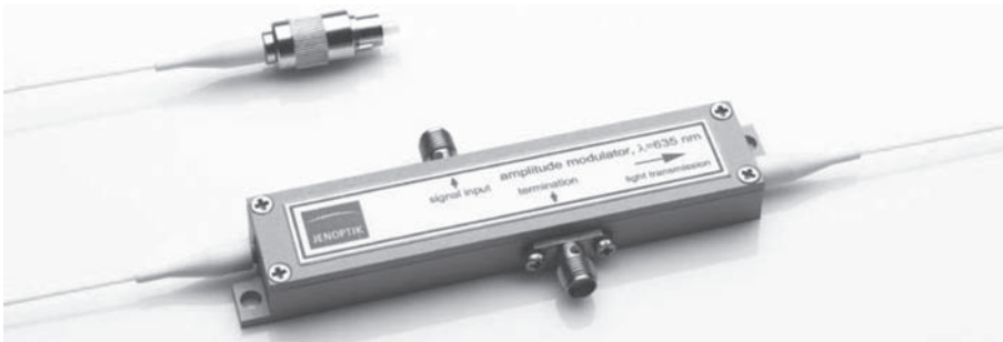
An \text{LiNbO}_3 -based Mach-Zehnder amplitude modulator for use from the visible spectrum to telecom wavelengths, with modulation frequencies up to 5 GHz. This particular model has V_{\lambda/2} = 5 \text{ V} at 1550 nm. (© JENOPTIK Optical System GmbH.)
