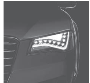
The Audi A8 uses LEDs for nearly all its lighting, including headlights. (Used with permission of Audi of America, Inc.)
