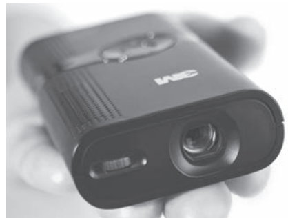
A handheld microprojector MPro120 from 3M for projecting photos and videos on a wall uses LEDs for its projection light. (Courtesy of 3M.)
