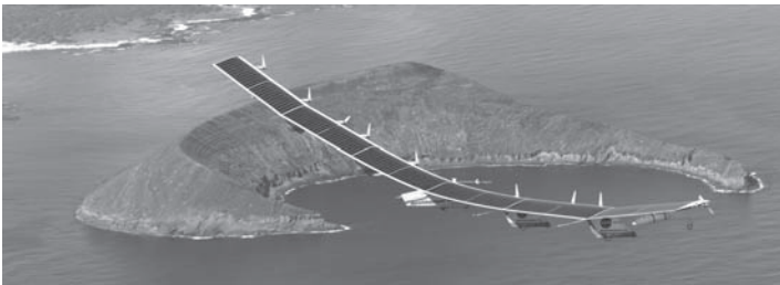
An experimental solar cell aircraft called Helios flying over the coast of Hawaii. (Courtesy of NASA Dryden Research Center.)
