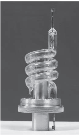
Theodore Maiman's ruby laser. The helical xenon flash surrounds the ruby crystal rod (an \text{Al}_2\text{O}_3 crystal doped with \text{Cr}^{3+} ions) and provides optical pumping of the chromium ions in the ruby rod. (Courtesy of HRL Laboratories, LLC, Malibu, California.)
