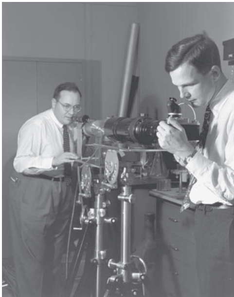
Arthur L. Schawlow is adjusting a ruby optical maser during an experiment at Bell Labs, while C.G.B. Garrett prepares to photograph the maser flash. In 1981, Arthur Schawlow shared the Nobel Prize in Physics for his "contribution to the development of laser spectroscopy." (Reprinted with permission of Alcatel-Lucent USA Inc.)
