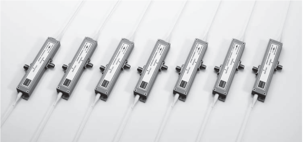
Fiber-coupled phase and amplitude modulators. The Pockels effect in lithium niobate is used to modulate the refractive index and hence the phase of an optical signal. In amplitude modulators, the Pockels effect is used to modulate the refractive indices of the two arms of a Mach–Zehnder interferometer, and hence the optical output. (© JENOPTIK Optical System GmbH.)
