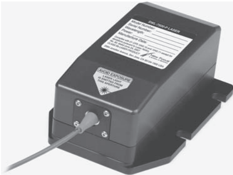
A commercial external cavity diode laser using the basic principle shown in Figure 4.51 (U.S. Patent 6,556,599, Bookham Technology). The output is a single mode at 785 nm ( \pm 1.5 pm) with a linewidth less than 200 kHz, and coupled into a fiber. The output power is 35 mW, and the SMSR is 50 dB. (ECDL, SWL-7513-P. Courtesy of Newport, USA.)
