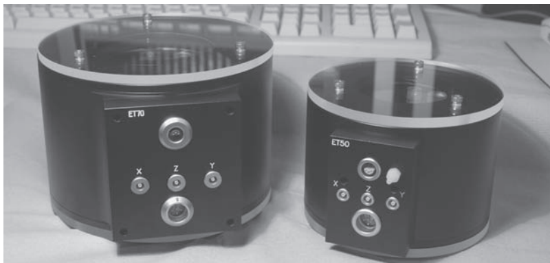
Piezoelectric transducer controlled Fabry–Perot etalons. Left has a 70 mm and the right has a 50 mm clear aperture. The piezoelectric controller maintains the reflecting plates parallel while the cavity separation is scanned. (The left etalon has a reflection of interference fringes on its surface plate that are actually on the adjacent computer display; not shown.) (Courtesy of IC Optical Systems Ltd.)
