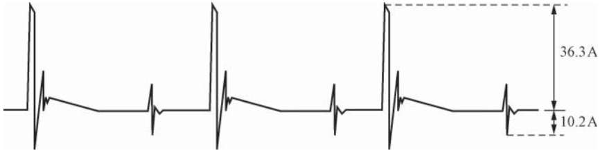
Figure 9.33 Secondary current waveform ( R_o and C_o connected)
