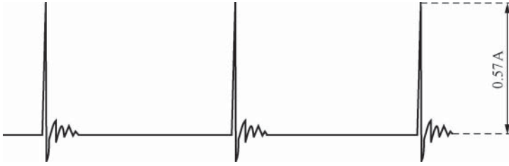
Figure 9.28 Primary spike current waveform
