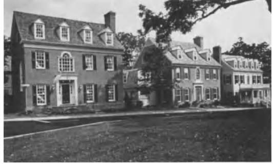
Figure F-3. At Kentlands, the urban regulations require otherwise typical suburban houses to conform to a build-to line, and limit automobile access to private lots from rear alleys.
