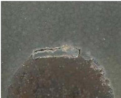
Figure 14. Penetrated casting surface due to MEP.
