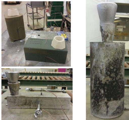
Figure 1. Tested ExOne molds and the cast bar and cylindrical geometries.
