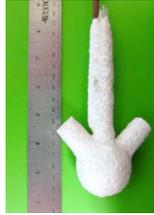
Fig. 1. The spherical ceramic shell mold used for the quenching experiments.
