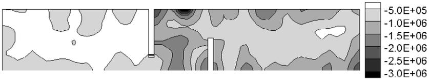
Figure 4. Predicted minimum instantaneous acoustic pressure (Pa) in domain for a configuration with baffles separated at a distance of  $1.0 \lambda$  for water along the central x plane.
