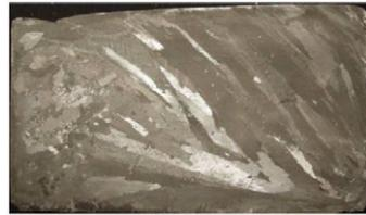
Figure 4. Macrostructure of the solidified Sn-3 wt.%Pb [13].
