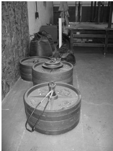
7.1 Heavy weights are used in static load, drop and repetitive cycle testing to verify the strength and durability of benches. Photo credit: Bill Main
