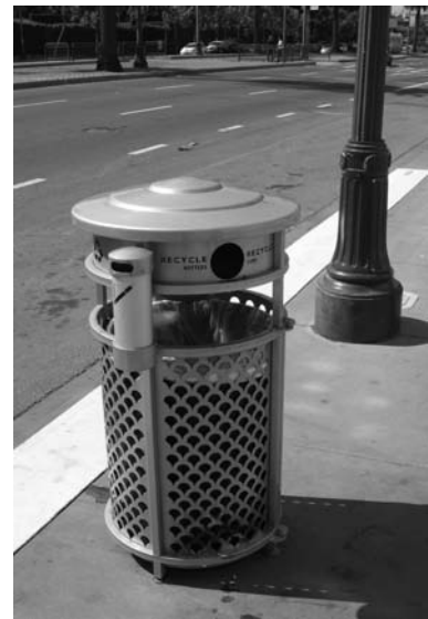
5.14 This San Francisco litter receptacle has a place in the top for bottles and cans to discourage folks from going through the trash to retrieve recyclables. Photo credit: Bill Main
