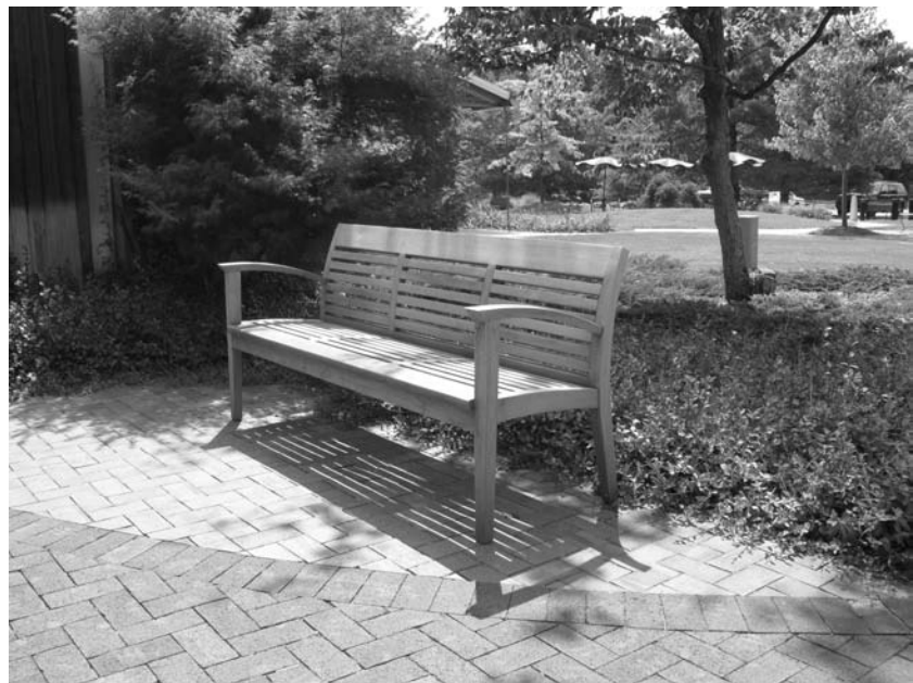
8.3 An example of a bench that conforms to ADA dimensional requirements. It has clear space for a wheelchair next to it. Photo credit: Bill Main
