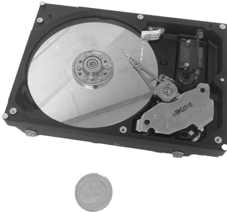
Figure 12.1: A partially-disassembled magnetic disk drive.
