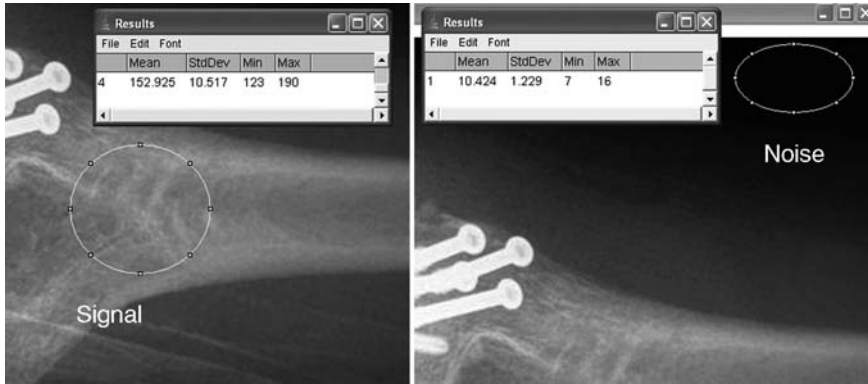
Fig. 5.8 A simple estimate of Signal to Noise Ratio (SNR) in an X-ray image. The Signal is measured as the average intensity in a selected region of the anatomy, in this case the base of the humerus, and the Noise in a region of the image where there is no signal from anatomy. We can then calculate (using Eq. 5.10) that, for the base of the humerus, the SNR is 0.66 \times \frac{152.9}{1.23} = 77.6 . Obviously, this method of measuring SNR is highly dependent on where in the image the signal is measured and it takes no account of the importance of contrast (the ‘Results’ windows are the output of the ImageJ Menu: Analyze > Measure command applied after drawing the ROI)
