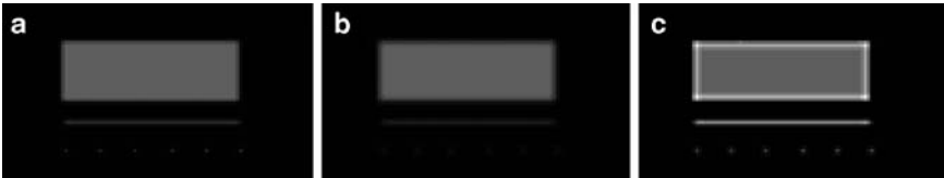
Fig. 7.37 Application of a smoothing filter prior to the high boost filter. (a) Original image. (b) Smoothed original. (c) High boost applied to image b. In comparison with Fig. 7.36 the point features, which simulate noise, are much less strongly enhanced
