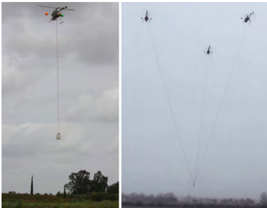
Fig. 3 Single and multiple UAV slung load transportation.
