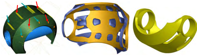
Fig. 10 Design space and FE model (left), design proposal as results of the topology optimization for a lightweight design (middle) and CAD implementation of the cap (right).
