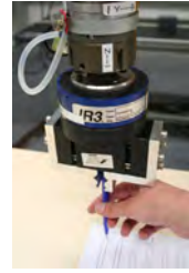
Fig. 6 The user grabs the pen and moves the robot.
