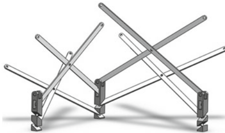
Fig. 2 CAD model of the two-dof deployable unit
