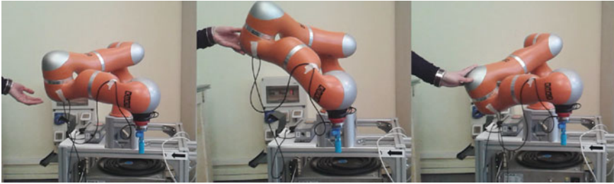
Fig. 4 From left to right , the first image represents the robot configuration when redundancy is not exploited, the second and the third images represent other two possible configurations, elbow up and elbow down respectively
