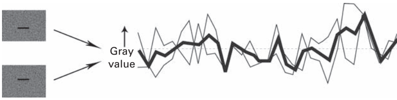
Figure 6.1 Noisy CT images of a water phantom, with a profile from each (solid lines) and the mean of the two profiles (thick solid line).
