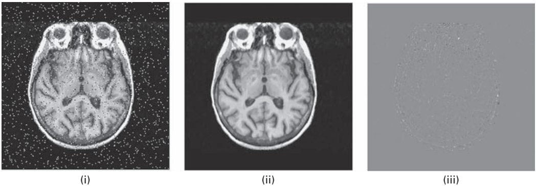
Figure 8.9 (i) A 256 \times 256 image with salt-and-pepper noise (identical to Fig. 8.2(i)). (ii) The effect of convolution with an adaptive median filter (using a multiple (see text) of 1.0). (iii) The difference between the image in (ii) and the image in Fig. 8.2(ii).
