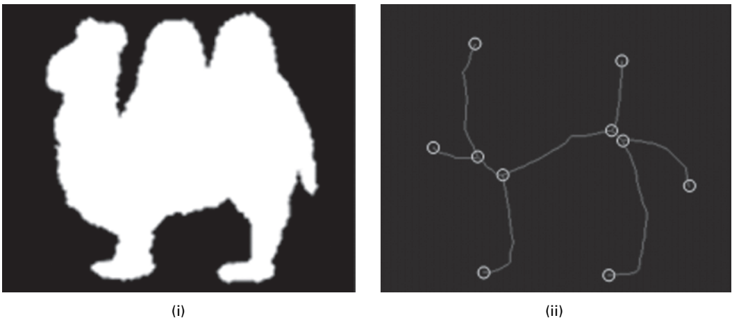
Figure 11.3 (i) Image and (ii) its skeleton (red), with its branch points (white) and end points (green) circled. See also color plate.
