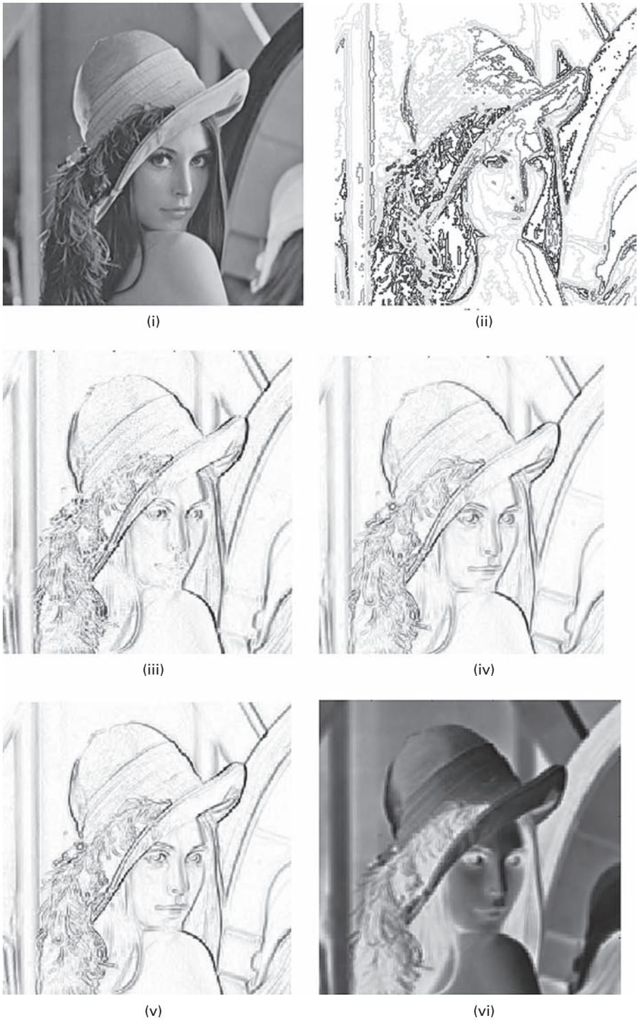
Figure 6.30 (i) Original (noiseless) 256 \times 256 image and (ii) its contours. Results of gradient edge detection using (iii) Roberts, (iv) Prewitt, (v) Sobel, and (vi) Frei-Chen operators. See also color plate.
