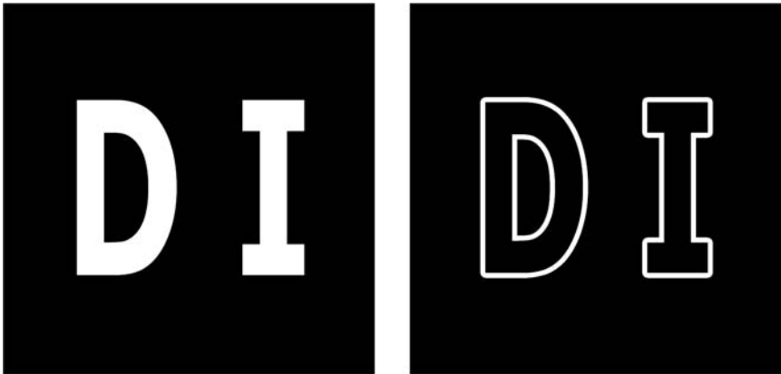
Figure 6.27 Repeated subtractions performed on the pixels of the image on the left result in the image on the right.
