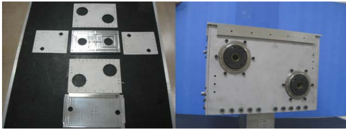
Fig. 10. Mechanical parts (LHS) and assembled (RHS) actuation module unit
