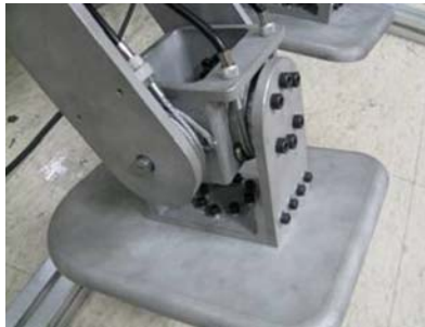
Fig. 8. Photo of realized ankle module in a BK leg mechanism
