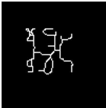
(b) Generalized Voronoi Diagram obtained from the coarse map.
