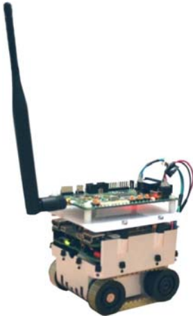
Fig. 12. Prototype: BeBot combined with nanoLOC Development Board
