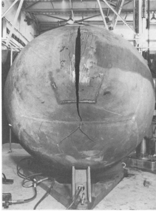
Figure 8 Sphere Ø 1800 (n° 2) after Failure
